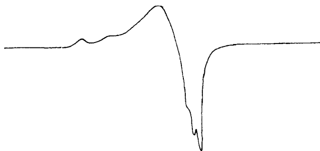
Figure 5 EPR spectrum of the Cu(II) complex of the sodium salt of 4 mol % NNMBA-crosslinked PAA.
